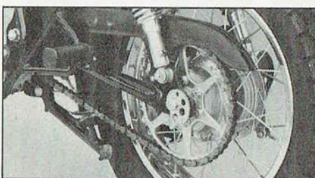
Like the dual purpose XT250, the Exciter I has snail chain adjusters and a lightweight rear sprocket.
