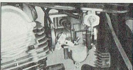
Not all parts of the Exciter I will appeal to beginning motorcyclists. The choke knob mounted on the carb is difficult to reach.
