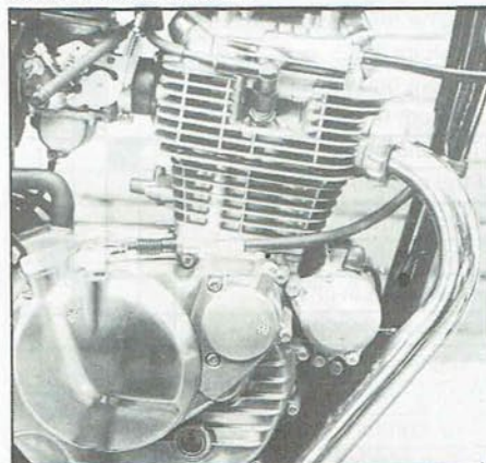
The LTD motor produced more midrange torque than either of the others. It was the most reliable starter, too.
